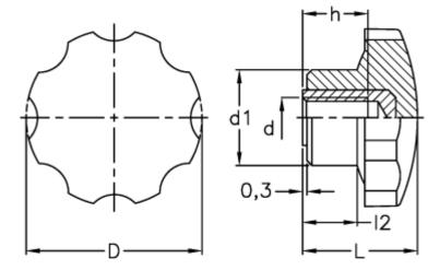
$$\begin{array}{ll} D & = 25 \\ d1 & = 15 \\ d \ 6H = M5 \\ h & = 10 \\ L & = 18 \\ l2 & = 9 \end{array}$$
